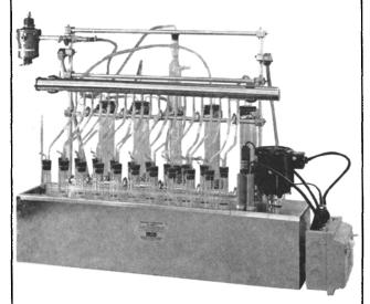
PRINCIPLE: Clean air is bubbled at a constant rate through the sample, maintained at constant temperature, until rancidity is developed. The aeration time to the inception of rancidity is recorded. The peroxide values of three sample portions which have been aerated separately are plotted against their aeration times. Keeping time, i.e., the time of aeration corresponding to a predetermined peroxide value for the organoleptic rancidity point, is read from the graph.
